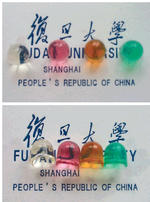
Figure 2. Photographs of ordered transparent mesostructured block copolymer-silica composites doped with transition metal ions of the peg-top column shape prepared by liquid-paraffin-medium protected solvent evaporation. Given samples are shown in (a) vertical view and (b) side view. The typical size of given samples is 0.9 cm high and 0.8 cm in diameter of the cross section. These monoliths show various colors in accordance with the corresponding slocation metal ions doped within them, which is colorless for pure silica sample, pink for \text{Co}^{2+} , yellow for \text{Fe}^{3+} , and green for \text{Cu}^{2+} (from left to right).
