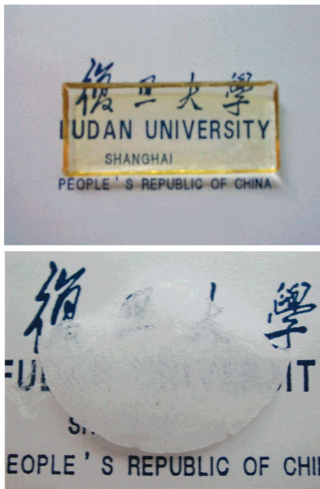
Figure 1. (a) Photograph of ordered transparent mesostructured block copolymer-silica composite prepared by liquid-paraffin-medium protected solvent evaporation. The given sample is 4.8 cm long, 2.1 cm wide, and 0.2 cm thick, crack-free, and optically transparent. (b) Photograph of mesoporous silica monolith after calcination, which is opaque perhaps due to microcracks inside.
